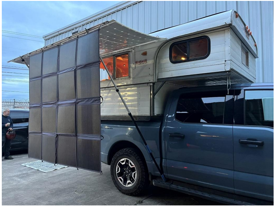
Matt Mortenson's vintage camper on his Ford Lightning truck is powered with marine grade solar panels and batteries.
