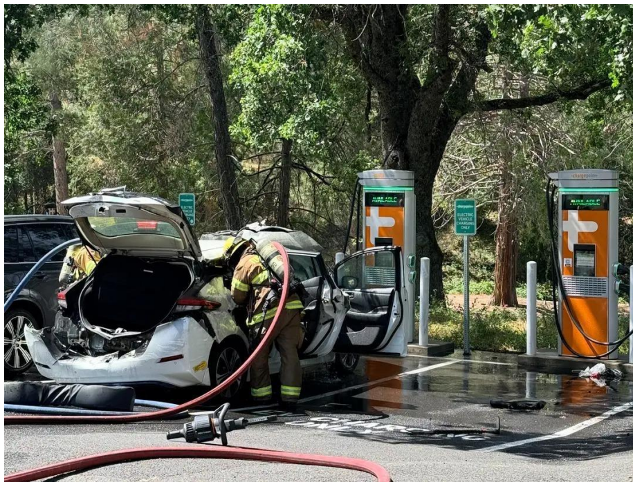
A Nissan Leaf with likely a faulty cell caught fire at a DCFC in California. Nissan has issued a recall affecting some 40,000 Leafs of certain VIN numbers from 2019-2022 for risk of fire due to cell defects that can manifest during DCFC. Photo by Bob M.
